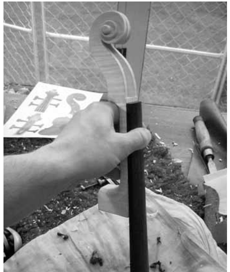
The scroll is carved with ever-decreasing chisel sizes.
