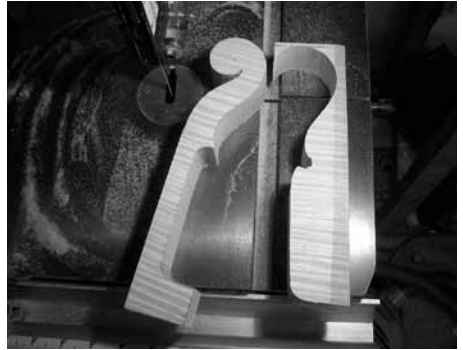
To carve the scroll, usually out of maple, first the outline is cut with a bandsaw.
