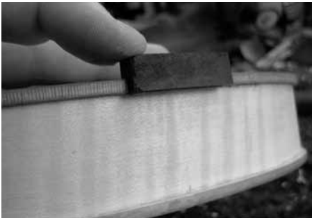
A preliminary bottom nut is shaped to help align the neck.
