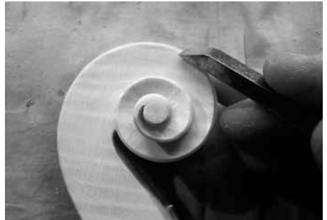
The scroll is carved with ever-decreasing chisel sizes.
