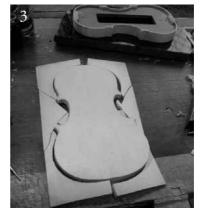
The top and back are then cut out with a bandsaw.
