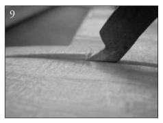
A double knife is used to cut the grooves, and then a very small special chisel removes the waste from between the cuts to a precise depth.
