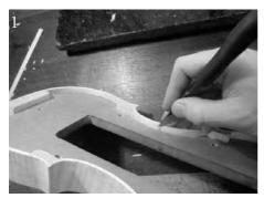
Linings, which are triangular-profiled slivers of wood, are glued to the inside of the sides to widen the gluing surface for the back of the violin.
