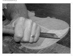
The outside arch of the back is roughed out to shape with chisels.
