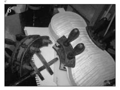
The front and back are spot glued to the sides.
