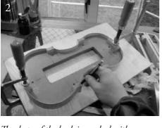
The shape of the back is marked with a special marker that draws a line an equal distance from the sides all the way around, after the central glueline of the back has been matched with the centre of the box.
