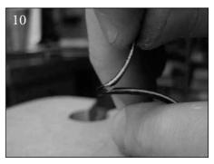
The front and back are removed from the sides by untacking the glue, and the six lengths of purfling with mitred joins at the corners glued in. With a tiny plane the scoop around the outside is shaped that connects the arch with the edge.
