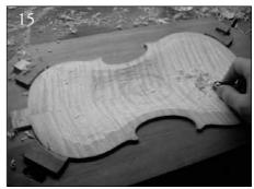
Then the inside arching must be prepared, again with chisels, planes and scrapers and precise measuring of thicknesses. These vary over the surface.
