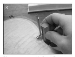
The next stage is to inlay the purfling. These are the fine black lines around the outside edge that provide some anti-splitting protection to the edges of the front and back surfaces, as well as adding to the instrument's attactiveness.
