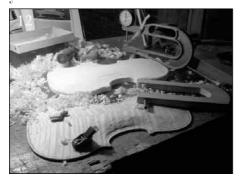
Now the outside arching is completed. The surface is finished with planes, then scrapers. Sandpaper clogs the pores of the wood and gives a dull finish.
