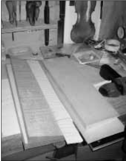
A set of wood for the body: Maple back on the left with strips of maple on top for the sides and spruce to the right for the top
