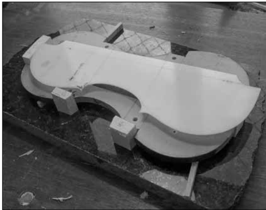
The template that determines the pattern sits on top, which has been used to create the mould that sits on a flat marble base. Some corner blocks have already been placed in position.
